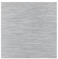
Brushed stainless steel is a modern and sleek material that will not rust. This material is very resistant to corrosion and is recomended if you want a bright metallic finish without a mirror reflection. The finished effect will create a bold, modern statementin your outdoor space. This material is food safe and safe for use with fire. It can be used indoors or outdoors. We can also offer coloured and textured stainless steel upon request for a truly unique finish.
