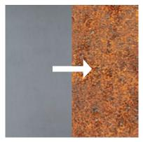
This metal generates a rust coating which will protect the inner material from corrosion. The material will weather naturally in the rain, creating a unique patina for every piece. It is best suited for outdoor use, as the rust colour can run into the surrounding area when wet. The rust can be carried by the rain and contaminate surrounding soil and make it difficult for plants to grow in the surrounding area.
