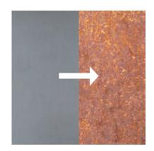
Mild steel, when left untreated, will rust. However, this material is not as long-lasting as Corten and will eventually rust through. This is a lower-cost alternative to Corten. This is best suited for outdoor use. The rate of deterioration is dependent on the conditions it is kept in, more rain will mean a shorter life span. The rust can be carried by the rain and contaminate surrounding soil and make it difficult for plants to grow in the surrounding area
