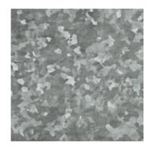
Galvanised steel is perfect if you are after an industrial look. This finish is achieved by dipping untreated steel into a protective zinc coating, to prevent rusting. This means that the material is durable and requires very little maintenance. Due to its zinc coating, we do not recommend this finish is used on products that will be in direct contact with food (it is perfectly safe on our tables with glass tops) or products that will be used to contain fire.
